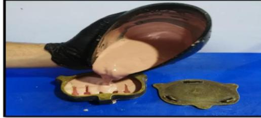
**Figure. 1 coating of mold by stone**
